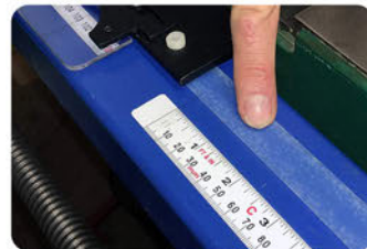
Applying tape to guide rails reduces friction
